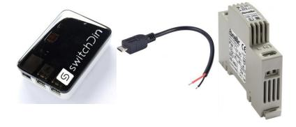
Option 2: Connection via a switchboard DIN mounted 240vAC to a 5vDC power supply using a micro USB connection lead, plugging the lead into the micro USB port of the Droplet. (DIN mount power supply and lead not included)
